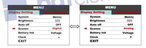
**8.5 Battery Ind**: Press UP/DOWN button to change the battery indicator, Voltage / Percentage / OFF.
