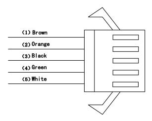
Brown wire : Anode(24v/36v/48V/52V/72V)
