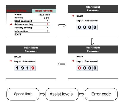
**8.11 Speed limit**: Press UP/DOWN will change speed limit, range 10km/h~60km/h.
