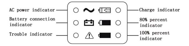
Trouble indicator: if it is over current error, the Charger will restart in 3-5 seconds. If it is over temperature error, the Charger will restart when the temperatures drop to the set value.
