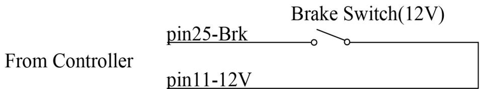
**Figure 9:** Wiring of brake switch(12V): 12V is provided by KLS-S controller on pin11
