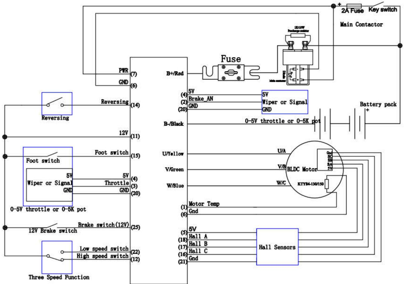
**Figure 7: KLS-S controller standard wiring(Three speed function control)**
