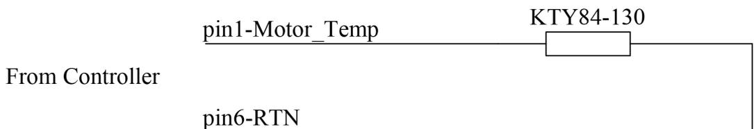
**Figure 10:** Wiring diagram for motor temperature sensor
