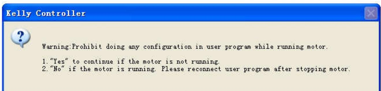
Anyway please try to do identification angle operation before running the motor. And please don't try to connect the controller to user program while the motor is still running, let alone change the setting in user program or Android App. That is to say, if you want to connect controller to user program or try to do programming, please stop the motor first.
