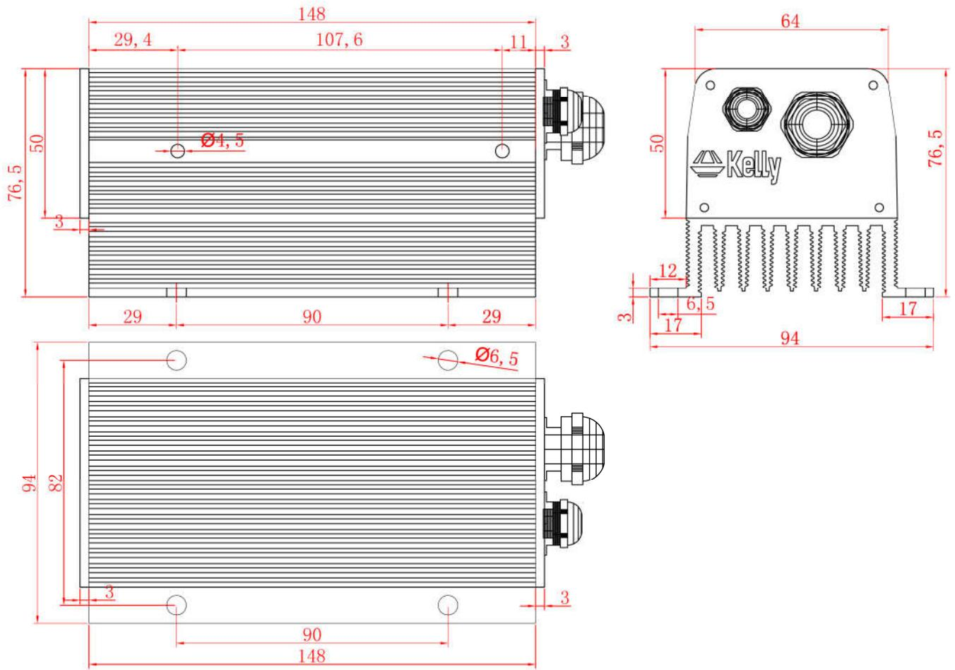
**Figure 2:**KLS6018S mounting holes' dimensions (dimensions in millimeters)
