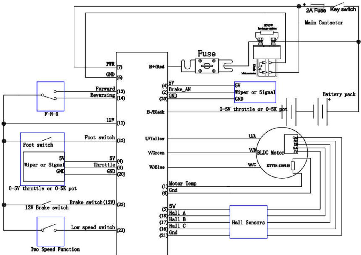
**Figure 6:** KLS-S controller standard wiring(F-N-R control)
