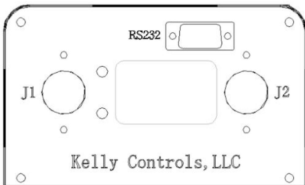
**Figure 4:** Back panel of HPM motor controller**Figure 5: The connecting diagram of J1 and J2**
